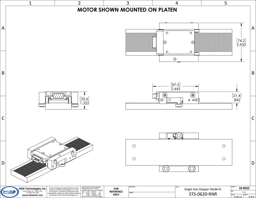
4 LINEAR STEPPER MOTOR SPECIFICATIONS Motor P/N **STS-0620-RNR** Continuous Force 6.0 lbs 26.7 N **Rated Current** 2.0 Amp Resistance/Phase @ 20C 2.40 ohms Inductance/Phase @ 20C 3.0 mH **Motor Phases Bearing Type** Roller Bearing Nominal Airgap 0.0015" **Motor Mass** 9.8 oz 279 grams Platen Mass 0.28 lbs/in 1.24N/in MOTOR POWER CONNECTOR
